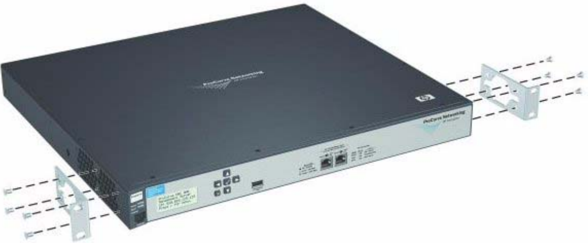
Figure 3. ProCurve NAC 800 with mounting brackets
