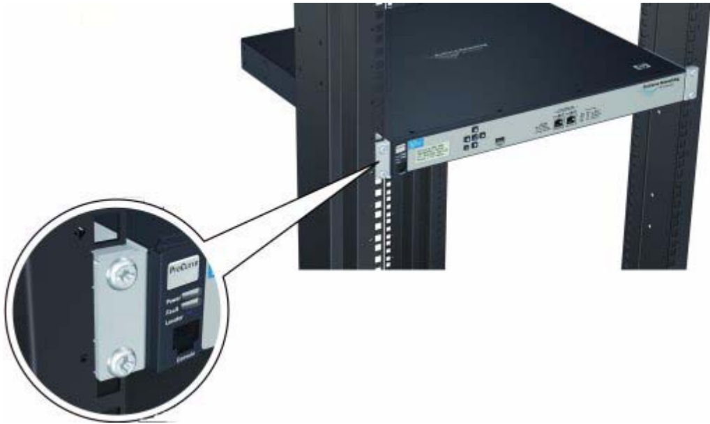
Figure 4. ProCurve NAC 800 rack mount example
